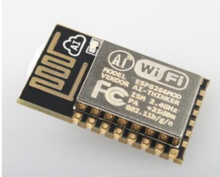
Figure 3 [Module Pin Counts, 22 pin, 16 mm *24 mm *3 mm]
